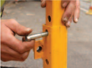
Ensure the holes in the inner and outer arm are aligned and insert locating bolt.
