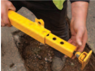
Slide inner arm inside outer arm to reach 'best fit' position for trench or excavation. PlateLOK has a max extension of 800mm.
